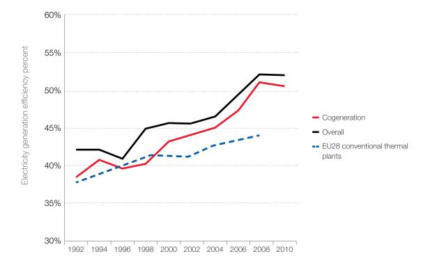
Refineries have long recognised the considerable efficiency gains offered by cogeneration, which now accounts for more than 90% of the electricity produced in EU refineries.
