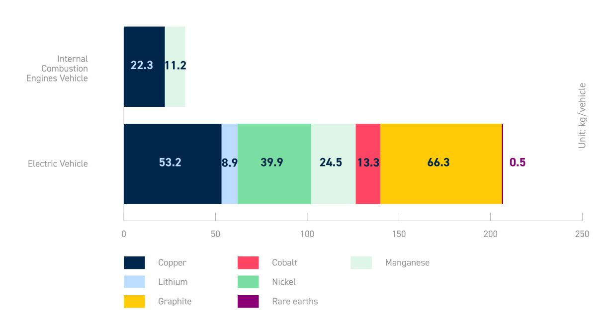
A typical electric vehicle (EV) requires six times the mineral inputs of a conventional car. Lithium, nickel, cobalt, manganese and graphite are crucial to battery performance, longevity and energy density, whereas rare earth elements are essential for permanent magnets that are vital for EV motors. The shift to EVs is set to drive a huge increase in the requirements for these minerals, meaning that the energy sector is emerging as a major force in mineral markets.
